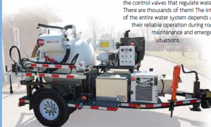
Garden City Park Water District's new Valve Turning Machine.
